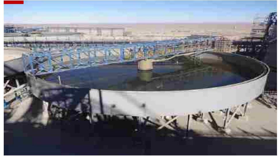
Concentrate thickener (max capacity 3,800 m3)
