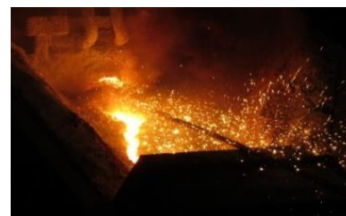
Copper outflow from the Flash Furnace
