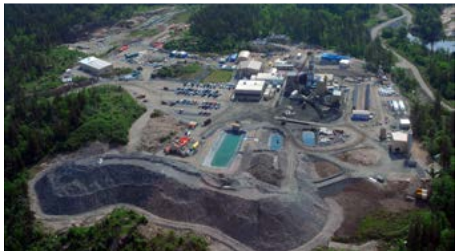
Waste rock temporarily stored on liner - Podolsky mine, Sudbury, Ontario, Canada
