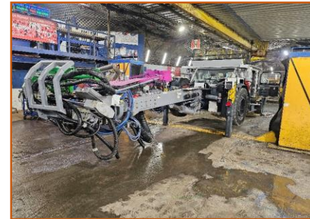
Prototype of an automated bolting rig
