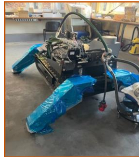
Prototype for cleaning boilers in the metallurgical plants
