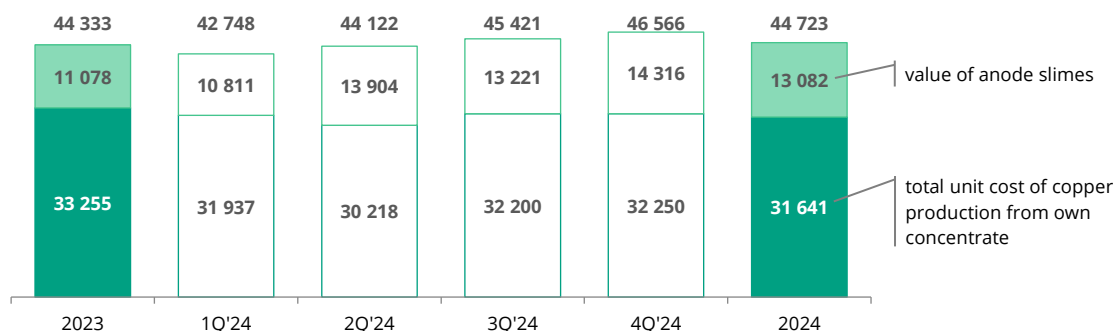
Chart 25. Pre-precious metals credit unit cost of electrolytic copper production – from own concentrate (PLN/t)
